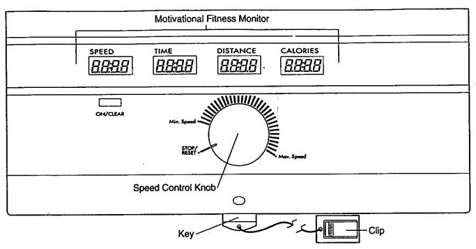
The heart of the treadmill is the innovative console. The console features a key-operated power switch, electronic speed control and four independent displays to provide continuous exercise feedback. Please read these instructions carefully before operating the console. Note: If there is a sheet of protective plastic on the face of the console, peel it off before operating the console.
